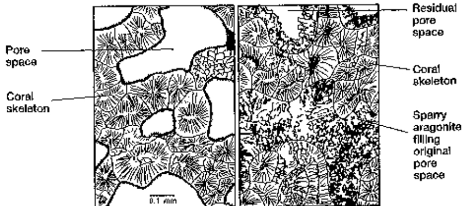
Fig. 1.2 Drawings from photomicrographs of: (a) a thin-section of skeleton cut from a living coral that has been diagenetically altered only by minute boring algae along the surface of the skeleton (producing the dark margin known as a micritic envelope); and (b) a coral, collected about 30 cm below the surface of a reef, in which aragonite cement has grown profusely into the interstices of the skeleton. From Friedman & Amiel (1974).
